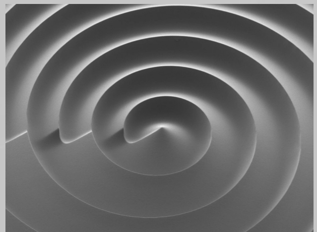
Fresnel Vertex Axicon with angles from 20°-45° with height of 10μm
