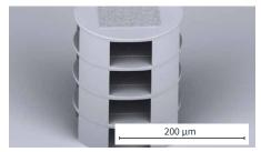
Stacked multilayer DOE structure with a pixel size of 550 nm x 550 nm.
