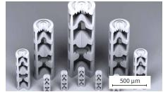
Lens stacks in different sizes, i.e. for biomedical applications/endoscopy.
