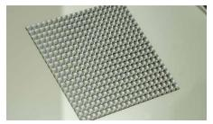
20 mm x 20 mm microlens array (MLA) with a filling factor of 100% consisting of 400 rectangular microlenses with dimensions of 1 mm x 1mm x 0,1 mm.
