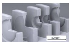
Horizontal lens system: Entire optical systems can be fabricated in a single process step without the need for alignment.
