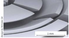
Mold (diameter 10 mm) with non-vertical sidewalls for micromechanical application. The mold was fabricated stitching-free using the IFoV Mode in combination with railroad hatching.
