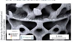
Bone-cartilage scaffold: 3D scaffold structures with Microfluidic reactor: Microfluidic structures with high micro- and macroporosity for bone cartilage implants. complexity and with tunable channel width.
