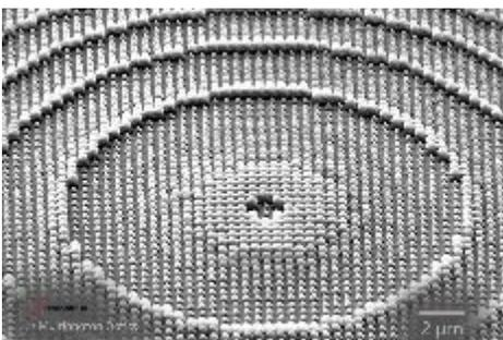
100 nm resolution: Metastructures with feature sizes below the diffraction limit can be fabricated in a single process step.
