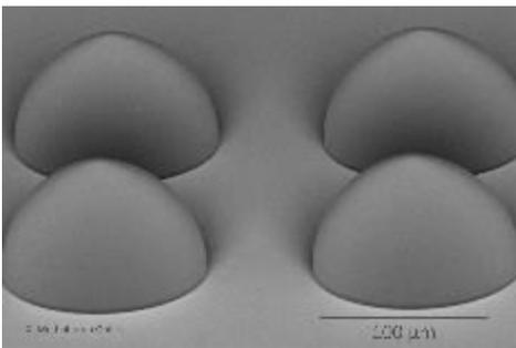
10 nm roughness: High quality microoptical elements with varying shapes (e.g. freeform) and sizes can be fabricated either on planar substrates or directly on active/passive devices.
