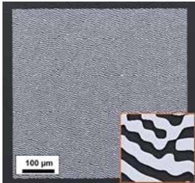
Reflective hologram (made with Au lift-off) consisting of 100 000 000 pixels and stitched from 50 μm write fields using an AFM correlation technique.
