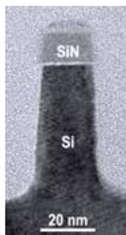
Silicon fins and trenches etched from PPA resist.
