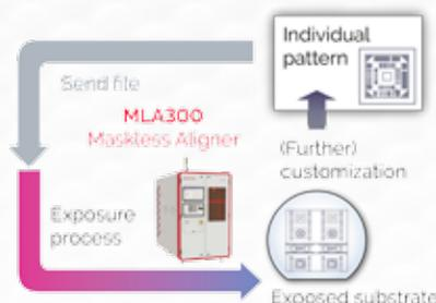
The benefit of Maskless Lithography is the inherent *rapid turnaround* and adaptation of the exposed patterns. Adaptations for customized products or even simply a large product portfolio no longer entail the time and cost of production and maintenance of an expensive mask set. Switching between product types is seamless, and does not require intervention to change masks.
