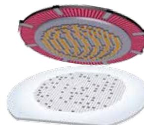
Tailor-made probe cards allow the testing of an entire wafer of computer chips in one go. In the production of these probe cards, the challenge lies in the alignment through very thick photoresists and the often *warped ceramic substrates*. MLA300 technology solves both problems through an increased travel range of its autofocus system up to 200 µm.
