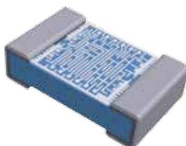
Electronic components are often produced on substrate materials such as ceramics which are selected for their robustness or thermal properties rather than surface quality. The Maskless Aligner technology flexibly follows surface warp and corrugations, increasing *uniformity and yield*. Process variations can also be compensated for *dynamically* by adjusting the exposed pattern.
