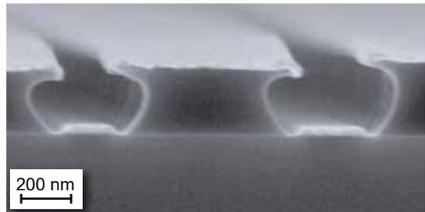
SEM view of a patterned bilayer resist with an undercut and evaporated metal before the lift-off
