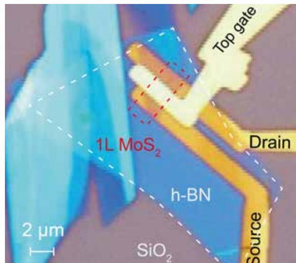
Left: A Hall Bar device on a single layer MoS<sub>2</sub> flake fabricated with the NanoFrazor and the bilayer lift-off. Right: Top-gated MoS<sub>2</sub> field-effect transistor with an h-BN top-gate dielectric and near-Ohmic electrical contacts.
