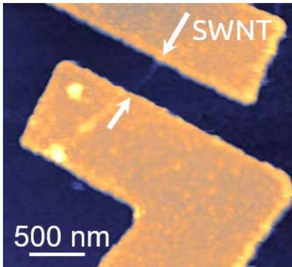
*A single-walled carbon nanotube contacted by two metal electrodes, which were patterned via the bilayer lift-off process. The in-situ overlay capability was used to detect the location of the nanotube.*
