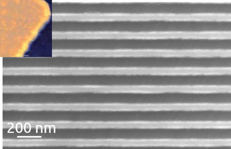
*70 nm half-pitch metal lines produced by the NanoFrazor and the bilayer lift-off process*
