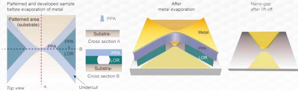
*Suspended PPA bridge geometry works as a shadow mask to create very small gaps.*
