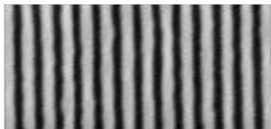
18 nm lines etched in 20 nm Au
