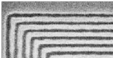
13.8 nm lines etched 65 nm deep in Si
