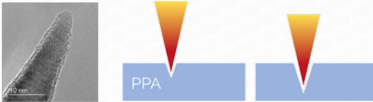
The NanoFrazor tip is extremely sharp (left) but due to its conical shape the patterning depth influences the pattern width (right).
