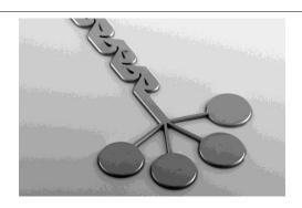
A master for a microfluidic mixer to be transferred by soft lithography in PDMS. The structure is patterned in 100  $\mu$ m Su-8 with the 375 nm laser wavelength of the MLA 150 Maskless Aligner.
