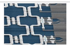
A SQUID magnetic flux sensor for Quantum technology Application after an 18 layers process made with the MLA 150 Maskless Aligner.
